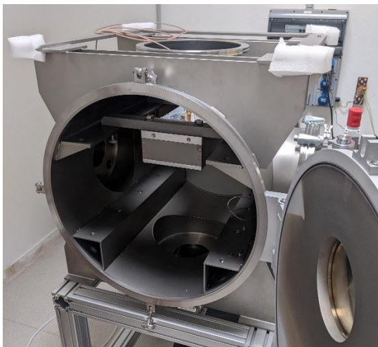
Images: (left) LPGP vacuum chamber for welding unit testing, (right) Salyut 7 on-orbit welding tests (1980s).
