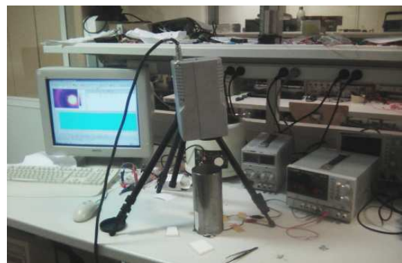
Photo 1: Delta Prime Heater temperature measurements with a thermocamera
