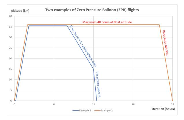
Fig. 1. Examples of zero pressure balloon (ZPB) flight altitude and duration.
